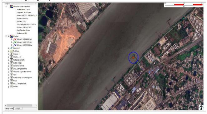
4. **Jet fire** from Full Bore Rupture of **MTBE** transfer pipeline with wind speed **5 m/s** and **D stability class** from jetty to terminal.
