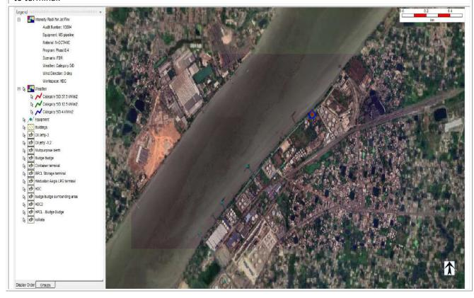
11. **Pool fire** from Full Bore Rupture of **MS** transfer pipeline with wind speed **5 m/s** and **D stability class** from jetty to terminal.
