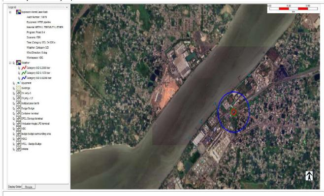
8. **Pool fire** from Full Bore Rupture of **Toluene** unloading hose with wind speed **5 m/s** and **D stability class** at Budge Budge Jetty-3.
