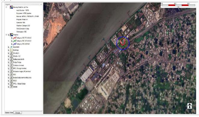
5. **Pool fire** from Full Bore Rupture of **MTBE** transfer pipeline with wind speed **5 m/s** and **D stability class** from jetty to terminal.
