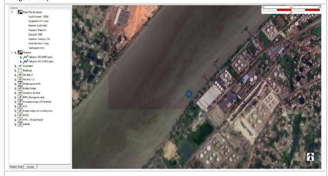
18. **Pool Fire** from Full Bore Rupture of **HSD** bunker hose with wind speed **5 m/s** and **D stability class** at Budge Budge Oil Jetty-1.
