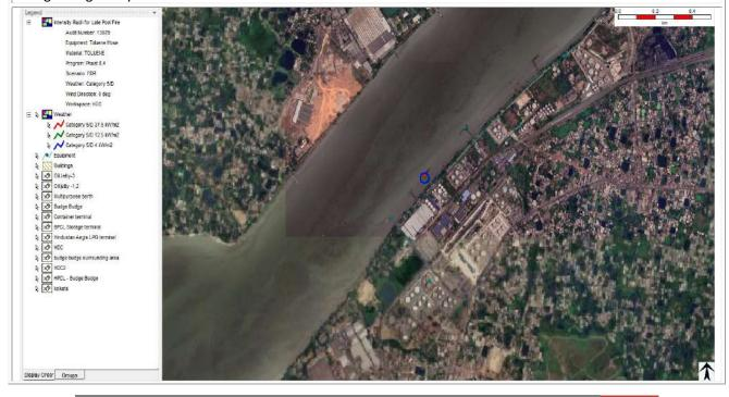
9. **Pool fire** from Full Bore Rupture of **Xylene** unloading hose with wind speed **5 m/s** and **D stability class** at Budge Budge Jetty-3.
