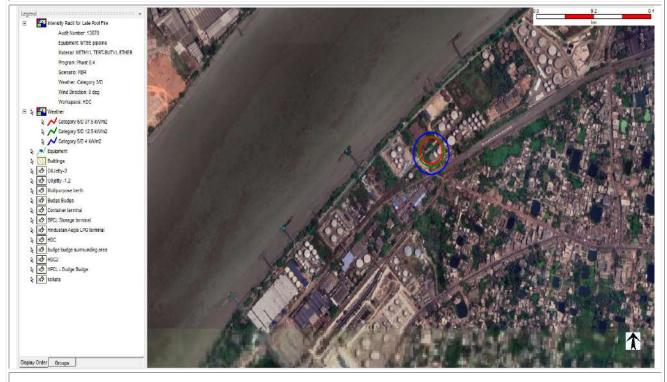
6. **Flash fire** from Full Bore Rupture of **MTBE** transfer pipeline with wind speed **5 m/s** and **D stability class** from jetty to terminal.
