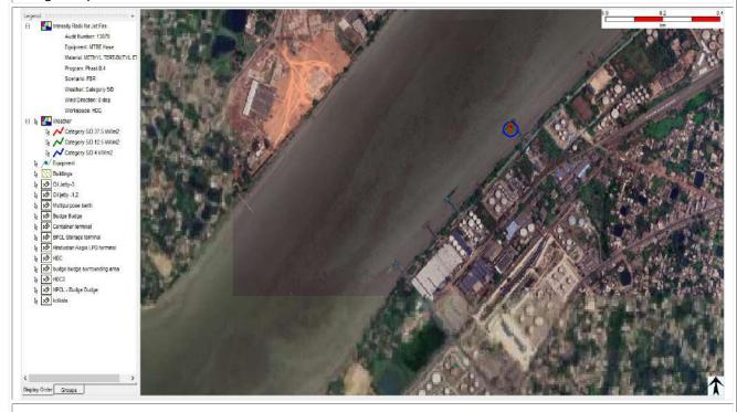
2. **Flash fire** from Full Bore Rupture of **MTBE** unloading hose with wind speed **5 m/s** and **D stability class** at Budge Budge Jetty-5.
