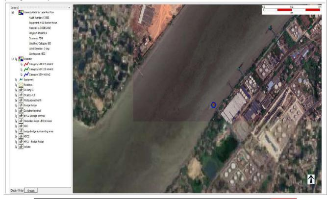
19. **Pool Fire** from Full Bore Rupture of **MS** transfer pipeline with wind speed **5 m/s** and **D stability class** from jetty to terminal.
