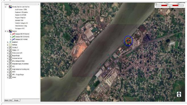
12. **Pool fire** from Full Bore Rupture of **Toluene** transfer pipeline with wind speed **5 m/s** and **D stability class** from jetty to terminal.
