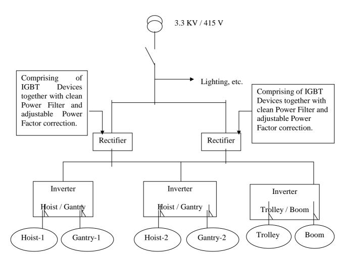
\* NOTE: 1 (one) Standby Inverter shall be provided for the 2 (two) Inverters for Hoist-1:Gantry-1 and Hoist-2:Gantry-2 while 1 (one) Standby Inverter shall be provided for the Inverter for Trolley-Boom. Suitable mechanism shall be provided for easy switch over to the Standby Inverters, as per requirement.
