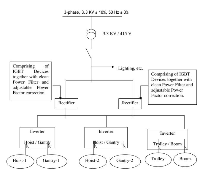
\* NOTE: 1 (one) Standby Inverter shall be provided for the 2 (two) Inverters for Hoist-1:Gantry-1 and Hoist-2:Gantry-2 while 1 (one) Standby Inverter shall be provided for the Inverter for Trolley-Boom. Suitable mechanism shall be provided for easy switch over to the Standby Inverters, as per requirement.
