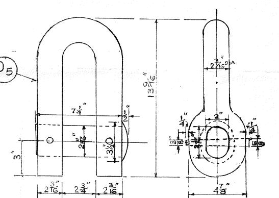
TEST LOAD- 55 TONS SAFE LOAD - 27-STONS 'D'TYPEJONANG SHACKLE
