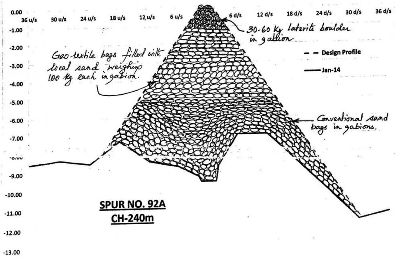
*Geo-textile bags filled with local sand weighing 100 kg each in gabion.*
