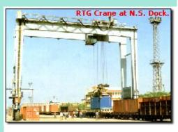
well as by Ships Cranes. Containers are moved to and from the stacking yard and stacked/unstacked at the container yard by rubber-tyred gantry cranes, prime-movers, reach stackers, etc.
